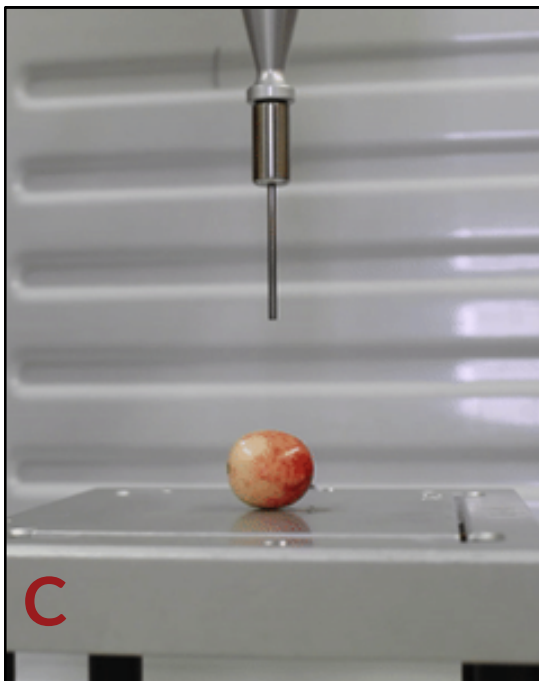
Cranberry fruit evaluated with double compression probe (A), chisel probe, puncture probe (C), and shearing probe (D).
